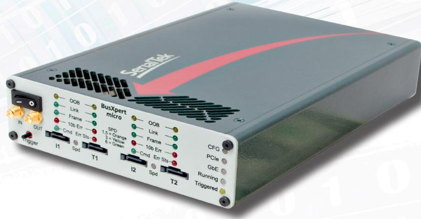
It is a 2 port 6 Gb/s analyzer that is also compatible with slower speeds and protocols. A 1 port model, licensed upgradable to 2 ports, is also available. SATA data rates of 1.5, 3.0 and 6 Gb/s are supported as are SAS data rates up to 6 Gb/s. Please also refer to the data sheets for the Pro II and Micro II versions of this analyzer. These newest models support data rates up to 12 Gb/s, 4 port configurations and trace buffer sizes up to 72 GBs.
