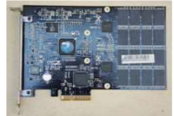
An OCZ Revodrive SSD, a full-height x4 PCI Express card
