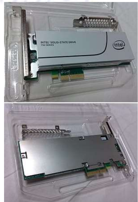
Intel SSD 750 series, an SSD that uses NVM Express, in form of a PCI Express 3.0 x4 expansion card (front and rear views)
