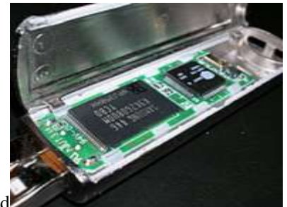
A disassembled USB flash drive . The chip on the left is flash memory. The controller is on the right.
