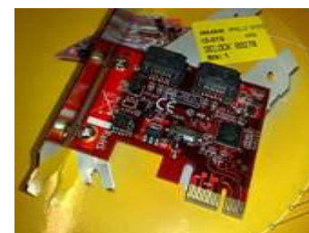
A Marvell-based SATA 3.0 controller, as a PCI Express x1 card
