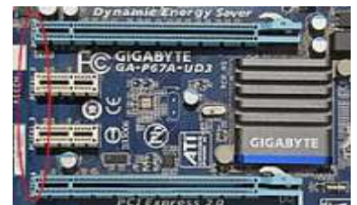
The PCIe slots on a motherboard are often labeled with the number of PCIe lanes they have. Sometimes what may seem like a large slot may only have a few lanes. For instance, an x16 slot with only 4 PCIe lanes is quite common. [6]
