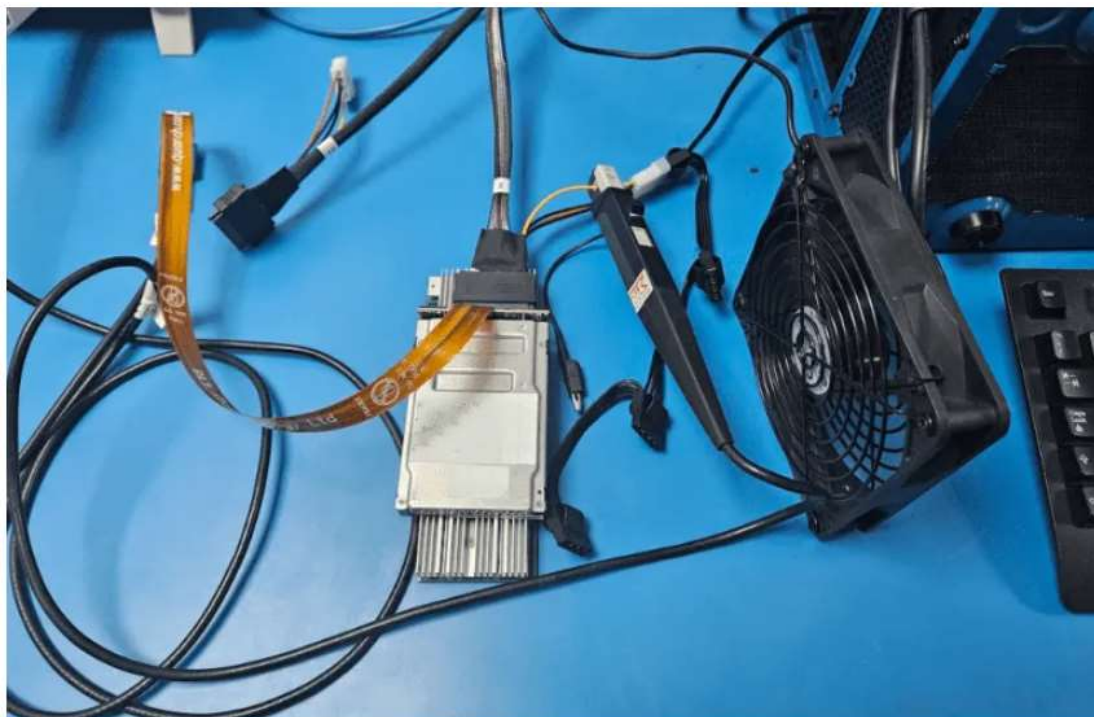
Gen5 U.2 SSD with Quarch PAM and current probe
