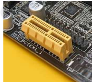
An open-end PCI Express x1 connector lets longer cards that use more lanes be plugged while operating at x1 speeds
