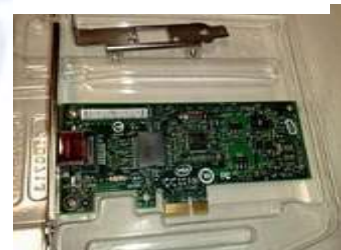
Intel 82574L Gigabit Ethernet NIC, a PCI Express x1 card
