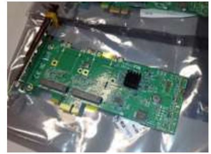
PCI Express x1 card containing a PCI Express switch (covered by a small heat sink ), which creates multiple endpoints out of one endpoint and lets multiple devices share it
