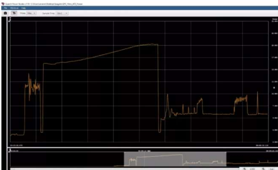
图 4-127 Quarch 2-channel PAM capture at 4uS then averaged to 10mS
