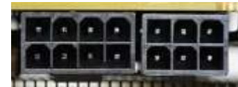
8-pin (left) and 6-pin (right) power connectors used on PCI Express card
