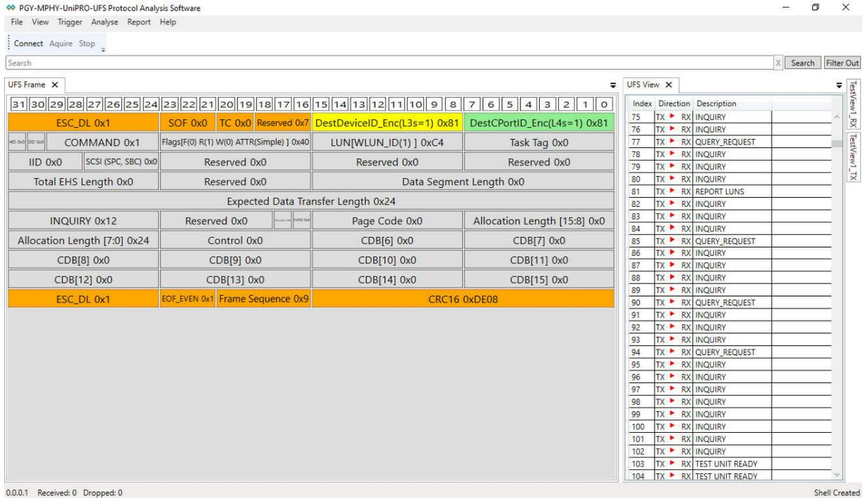
This view displays for information application layer transactions. UFS layer packets are listed and its packet level content.
