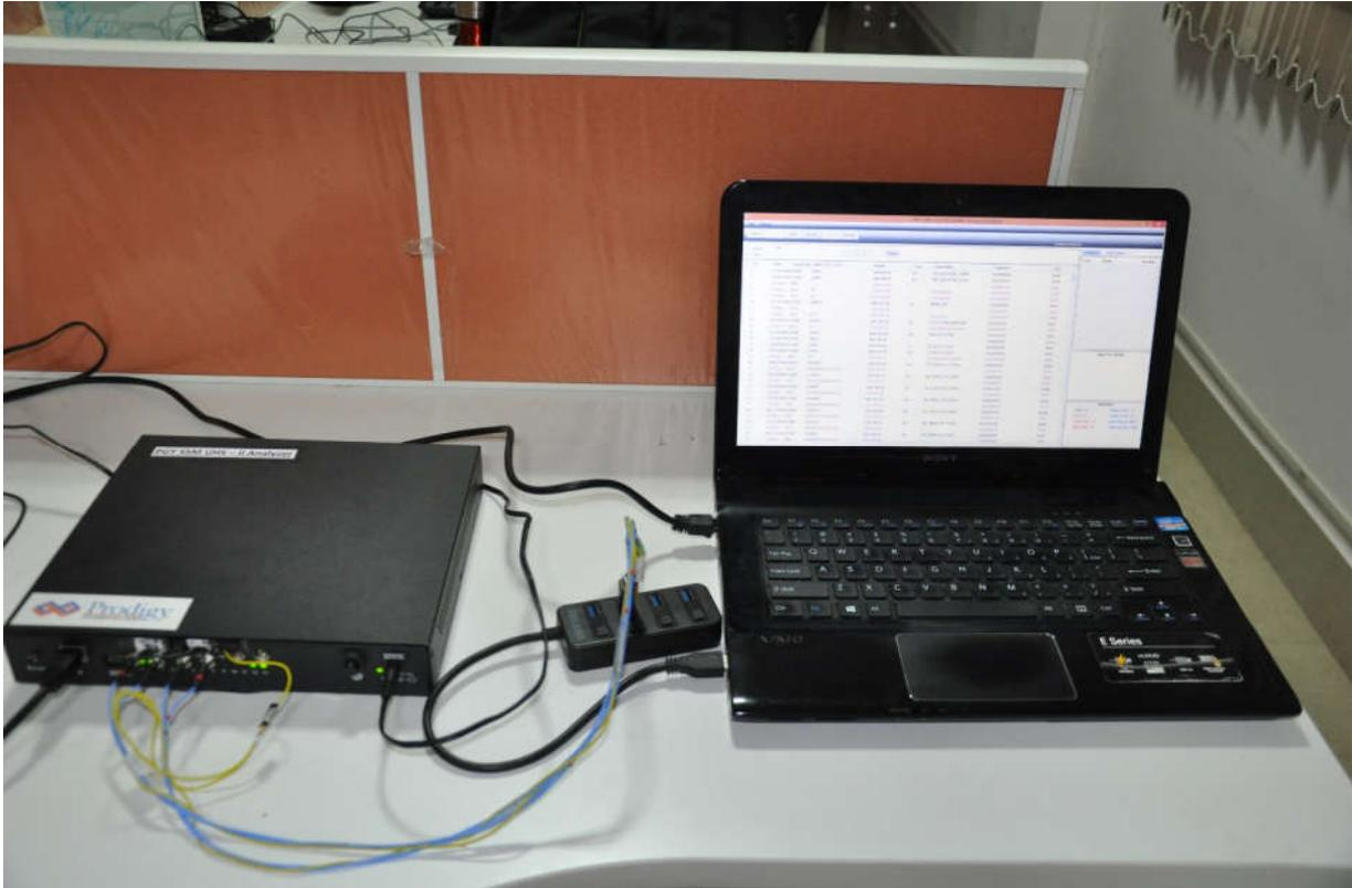
PGY-PMHY-UNI-PRO-UFS Protocol Analyzer provides USB3.0 and GBe interface for host connectivity. Software runs in host machine enables configuration of PGY-MPHY-UFS hardware for UFS protocol analysis including boot information capture for eMMC for comprehensive Protocol Analysis. High-speed host connectivity enables continuous streaming of protocol data and storage for long period of time.
